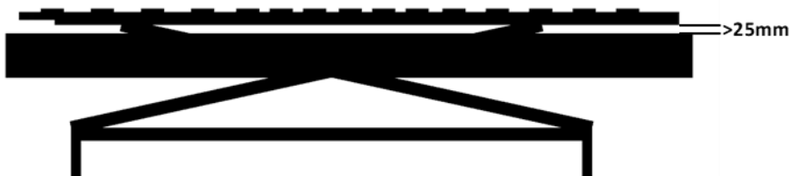
Figure 2: If the minimum distance between the bed frame and the bed panelling cannot be maintained, the lying surface may not be immersed in the bed panelling and may only be lowered to such an extent that there is a distance of at least 25 mm (= 2.5 cm) between the upper edge of the bed panelling and the lower edge of the bed frame.
